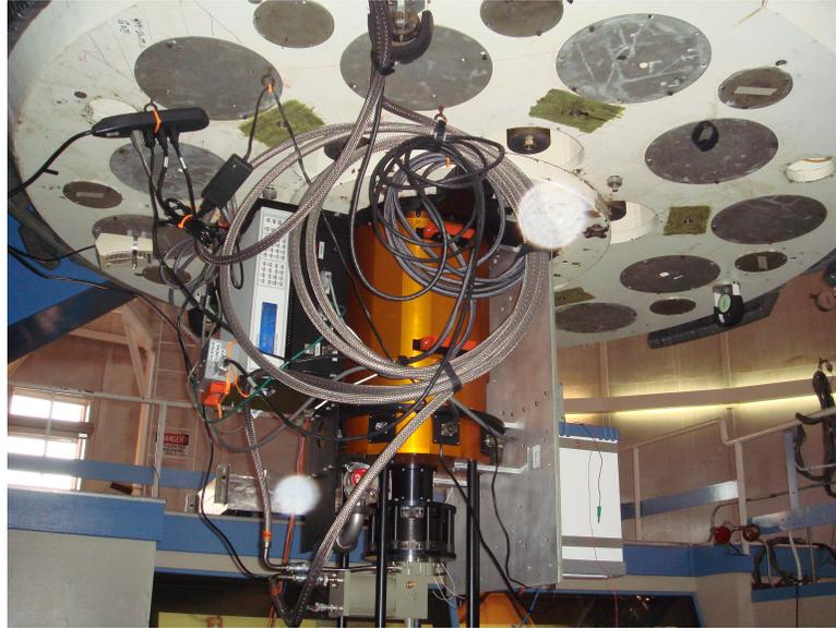
Figure 5.1: A photograph of the RIDL dewar mounted to the Kitt Peak 2.1m telescope.
